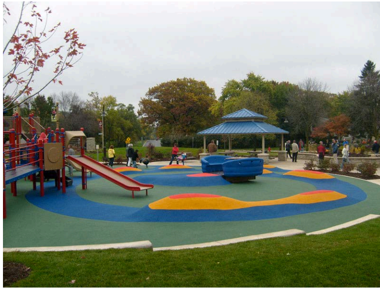
Figure 3. Poured in Place Playground Surface.
