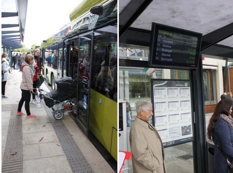
Bus stop, Trondheim. The stop is designed so the bus can stop close to the platform. High platform and buses with low floor allows for step free entry and exit.
